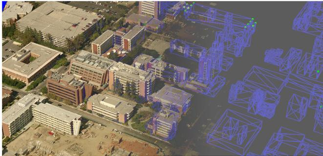
Figure 7. A textured 3D model for a university campus. The green points indicate the interactively marked correspondences between the geometry and the imagery, which were used for the recovery of the camera pose.
