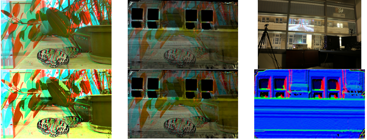
Figure 8: An example frame (from the video) used in Experiment #2. First column: (top) original frame, (bottom) adjusted frame. Second column: (top) projection of original frame on scene, (bottom) projection of adjusted frame on scene. Third column: (top) the projection onto the building’s facade; note the excessive ambient lighting present in the scene; distance over 20m, (bottom) the normal map of the projection surface.
