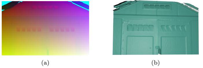
Figure 3: Experiment #1: (a) The XYZ map of the scene’s structure generated with SLS. (b) A render from a novel viewpoint of the reconstructed geometry.
