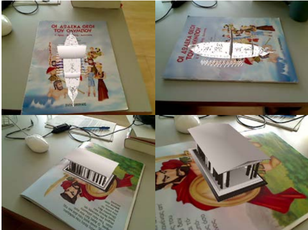
Fig. 3. Scenario I: Children book. The models placed in the captured frames vary according to the page's content. Model complexities: ship – 85200 polygons, Greek temple 4338 polygons.
