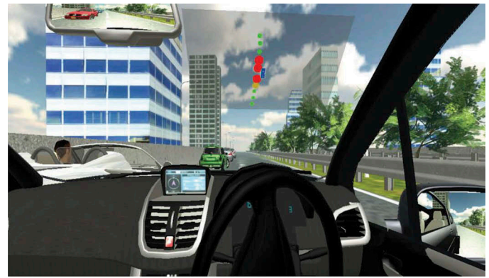
Figure 2. Driver VE view with the radar HUD depicting surrounding vehicles. The red circles are warnings about cars approaching on the left side.
